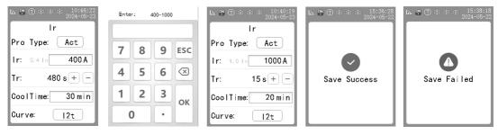
**Figure 28 Overload Long-time Protection Settings**
