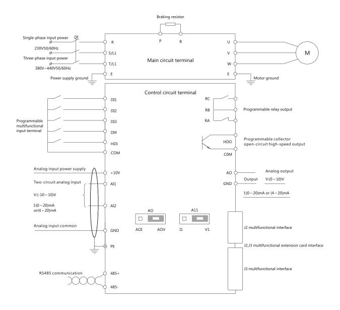
AO dip switch: Left position:  $(0\sim20)$  mA or  $(4\sim20)$  mA analog current output; Right position:  $(0\sim10)$  V analog voltage output. AI1 dip switch: Left position:  $(0\sim20)$  mA or  $(4\sim20)$  mA analog current input; Right position:  $(0\sim10)$  V analog voltage input. AI2: The current output needs to be customized.
