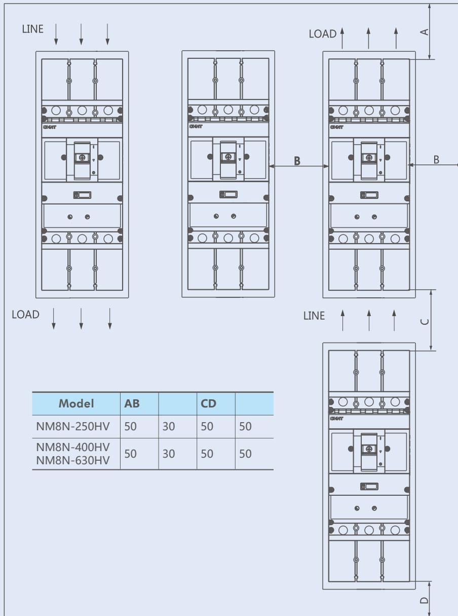
Minimum Mounting distance must be ensured.
