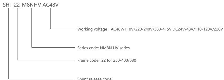
**Note:** Shunt release of 400/630A frame and 250A frame is compatible.
