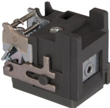
Shunt releases operate according to electrical signals, enabling remote control and automatic control of circuit breakers. When the supply voltage is equal to any voltage between 70% and 110% of the rated control power supply voltage, the shunt release should enable the circuit breaker to operate reliably.
