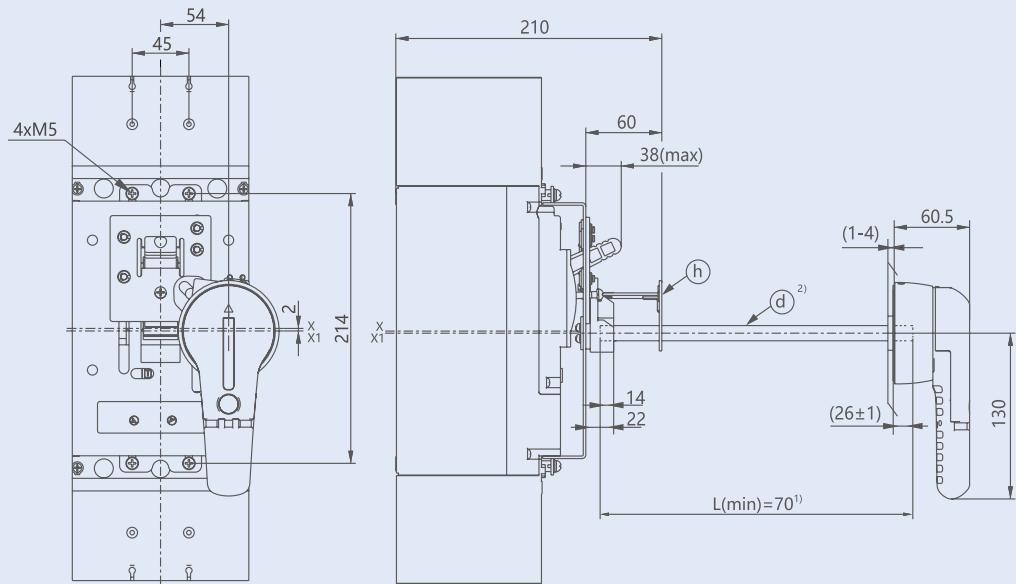
Note: 1) When  $L \geq 150$ , in order to avoid the shaft sagging, h support plate need to be installed; When  $70 \leq L \leq 90$ , support plate is not needed;
