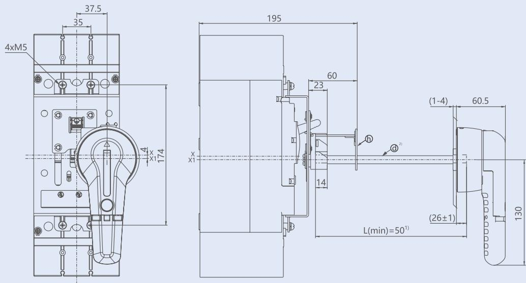
Note: 1) When  $L \geq 150$ , in order to avoid the shaft sagging, h support plate need to be installed; When  $50 \leq L \leq 90$ , support plate is not needed;
