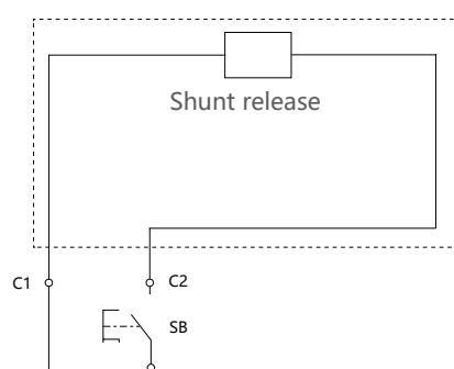
**Note:** When the rated control power supply voltage DC24V shunt release is used, the maximum length of the copper wire (each of the two wires) must meet the following table:
